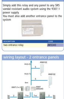
9307.2 timer for the lock release is required for each entrance unless a keypad is fitted in the panel
