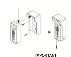
DO NOT OVER TIGHTEN the panel fixing screw
