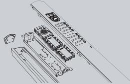
The composition of an audio or video door entry push-button column for Two Wire, Digibus or Digit 2 Wires systems requires the addition of an audio or video push-button electronic unit, and in some cases an additional push-button module type 12TS.
