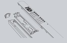
In order to assemble an audio or video column including call buttons, in systems with Sound System or A.C. call systems, add a speech unit or a video camera with a speech unit, name card illuminating LED art. R260 (one for every 4 push-buttons), and pushbuttons art. R200 or R200/50.
